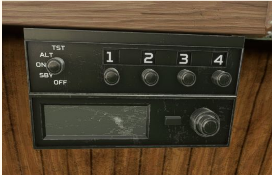
Radio stack: Transponder and VHF radio
